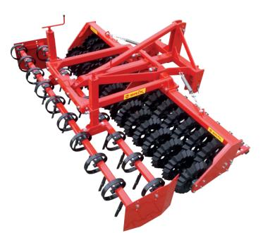
The two intermeshing polygon rollers with each 15 rings  $\emptyset$  450 |  $\emptyset$  550 mm (option:  $\emptyset$  550 |  $\emptyset$  550 mm) tend not to stick under the most extreme conditions either. The leading, 2-row harrow section (18 tine, thickness 45 x 12 mm) can be adjusted stepless in height by means of cranks.
