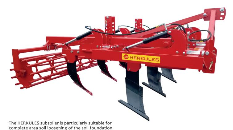
The trailing crumbler roller Ø 600 mm leaves a flat field. The oversized main frame profile tube 150 x 150 mm as well as the hydraulic stone protection (reduced price shear pin) ensure trouble-free operation. The rotatable, hardened tips as well as the divided, hardened wear plates can be changed very easily.
