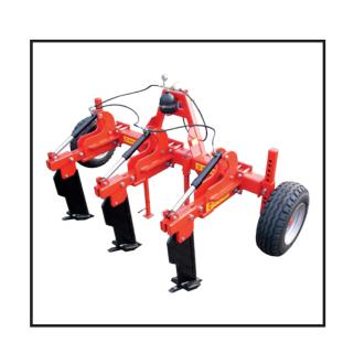
The support wheels 10.0/75-15 are the easiest and most inexpensive way to set the working depth.
